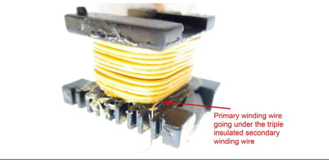
Note: In this case, the transformer provides critical double or reinforced insulation between the live parts and accessible parts.
